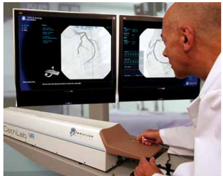
Figure 3. Catheterization laboratory simulator demonstrating coronary angiography. Reproduced by permission of Immersion Medical, Inc., Copyright © 2007 Immersion Medical, Inc. All rights reserved.
